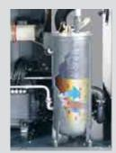
high-efficiency separation system. Most of the cooling fluid is initially separated from the air by centrifugal force in the separator tank. Any remaining fluid is separated by a 2-stage
