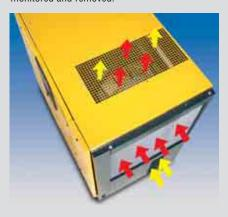
Cooling air for the motor and cabinet inside (shown by yellow arrows) is also drawn directly from ambient air and is exhausted through the same top exhaust opening. This allows easier ducting for heat recovery and energy management.
